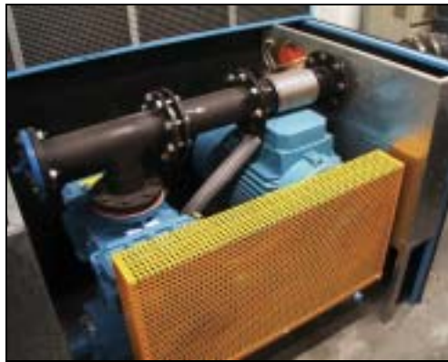
Fig. 2 Left: A Roots compressor is used as a flow generator Right: Microphones Type 4190 measure the radiated acoustic pressure
