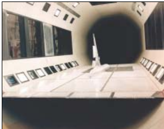
Fig. 10 DC-10 half model installed in the NASA Ames 12 foot pressure wind tunnel - the microphone array panel can be seen in the wall on the left
