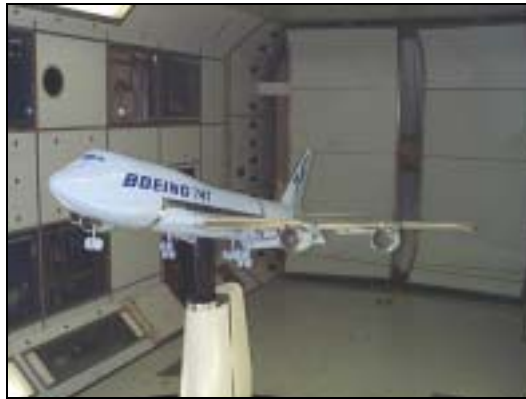
Fig. 3 Model of Boeing 747 installed in the QinetiQ (DERA) 5 metre pressurised low-speed wind tunnel at Farnborough, England
