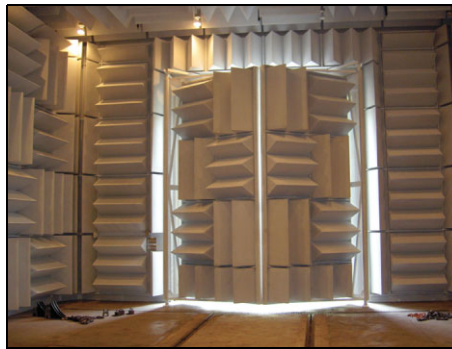
Fig. 4 Although the anechoic room is large enough to accommodate a full size truck, it can be effectively sealed against the influence of exterior noise sources
