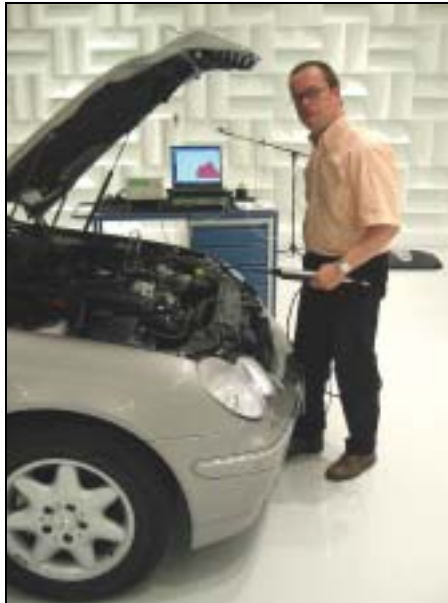
Fig. 2 Ulrich Heise is the NVH Development Manager at Benien. He is using Sound Intensity Probe Type 3599 to investigate noise sources from an engine
