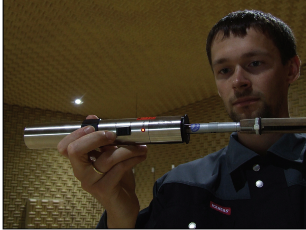
Fig. 1 An engineer performing the weekly pistonphone calibration
