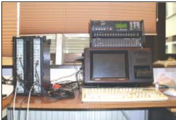
Fig. 5 ALSTOM Marine's PULSE system comprises two front-ends – a 5-channel and a 7-channel unit. They can either be used separately, or stacked together
