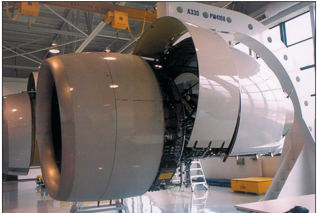
Fig. 1 A nacelle for one of the Pratt & Whitney PW4168 engines which power the A330 Airbus
