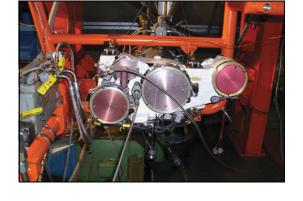
**Fig. 2** CH53 helicopter power transmission assembly Avio is also a leader in the sector of helicopter engines, developing and producing turbo-shafts and power transmission gearboxes for main rotor and the tail rotors.
