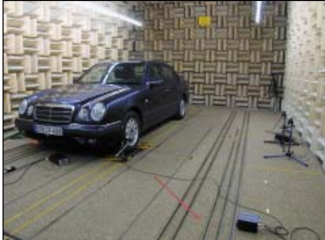
Fig. 4 An anechoic test cell at Pirelli
